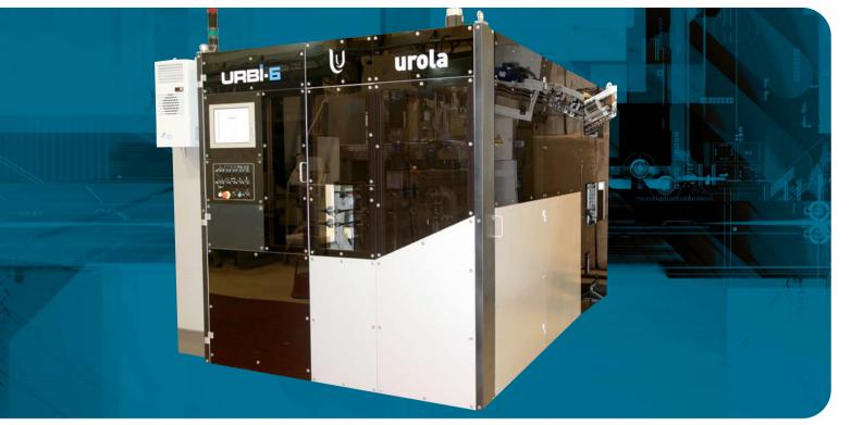
**URBI 6**, the new generation of UROLA's **ECO**machines, has 6 moulds in a linear configuration, capable of reaching a production in the region of 9,000 b/h. One of its key characteristics is its **very low carbon footprint**, offering the following **RELEVANT CHARACTERISTICS**.
