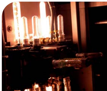
Preform Heating Oven, with minimum distance between preforms, and with wide homogenisation area.
