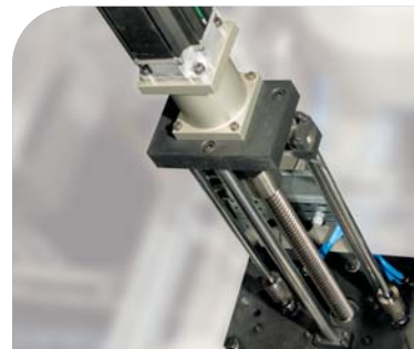
Preform stretch system, by means of servomotor.
